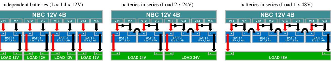
\*In case of connecting in series batteries, it is necessary to insert a bypass diode which protects the battery charger if the battery has an open element, preventing any current passing through the device. The model and sizing of the diodes must be evaluated based on the electrical characteristics of the load.
