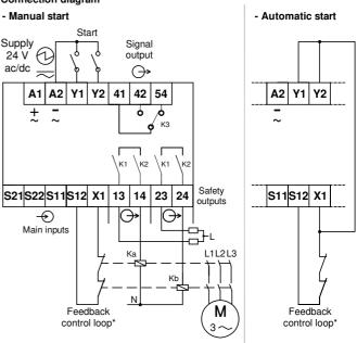
\* If it is not necessary to control the NC auxiliary contacts of the relays via a feedback loop, short-circuit terminals S12 and X1.
