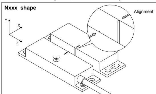
Fig. 1 Sensor alignment
